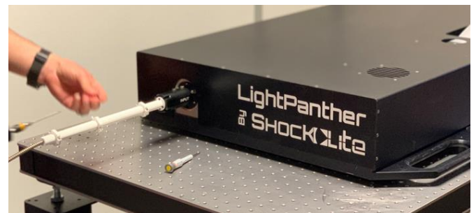
Figure 4 : The fiber injection module named the LightPanther
