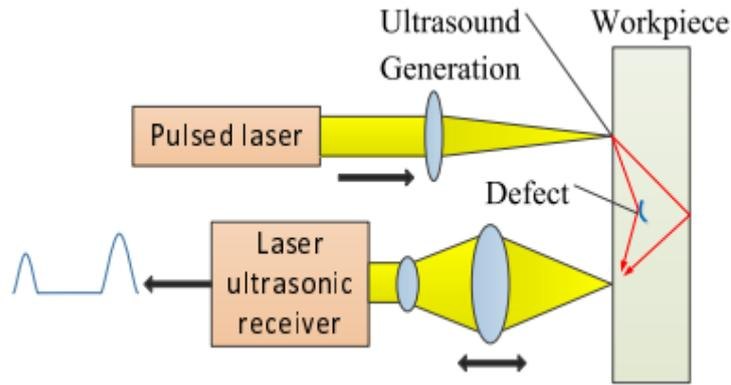
Figure 2 : Laser ultrasonic crack detection principle [2]
