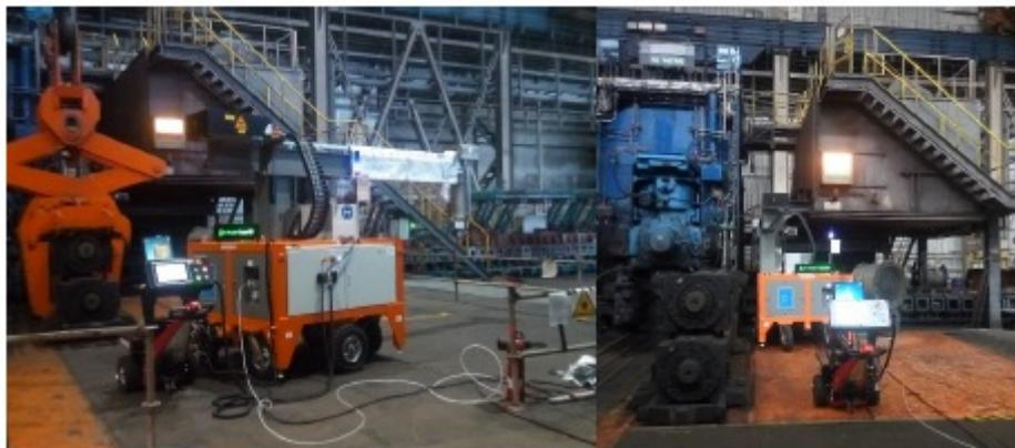
*Figure 6 : Laser Ultrasonics apparatus in industrial conditions (ArcelorMittal's factory in*
